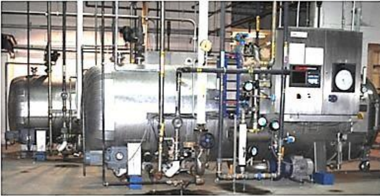
(4) Steam-Water Spray FMC retorts
